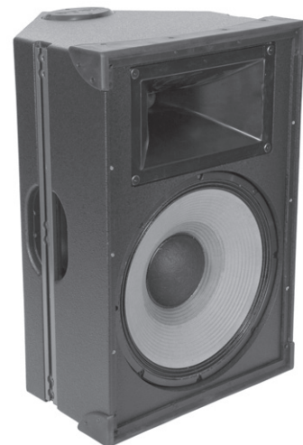
NT59 2 pásma full range, 15" + 1,4", 1 000 W + 500 W, 133 dB max, Gunness Focussing DSP™
