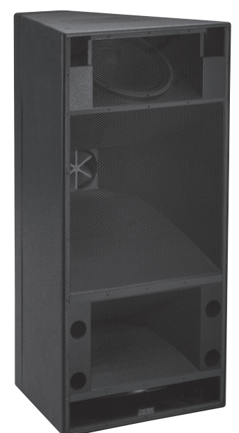
EAW MQH1346e 3 pásma full range VA4 systém, 2×15" slot-loaded + 10" horn + 2", 600 W/92 dB + 600 W/94 dB + 400 W/110 dB + 150 W/109 dB, quadamp.
